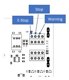
These outputs are open-collector type. They can be activated by settings in the CNC.INI file. The settings can be found under the section [GPIO\_RULES], below is an image showing a part of this.
